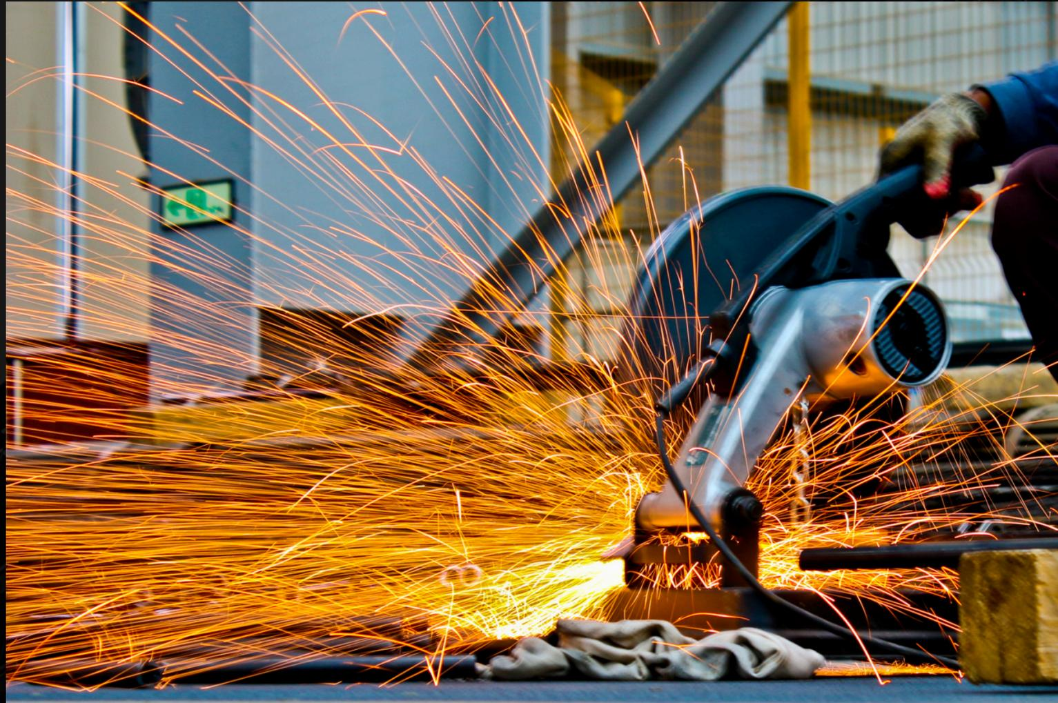
Grinding or striking materials can create flying object hazards.
